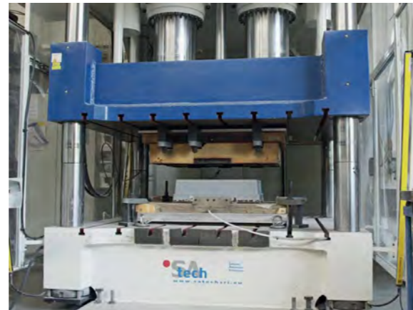
SMC moulding press.
