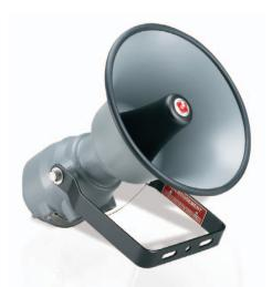
SSTX3-MV is an economical yet explosion-proof electronic siren capable of producing three high decibel tones from the same unit. The integrated circuitry is contained in a rugged die cast aluminum housing. The unique threaded rear access cover eliminates traditional time consuming bolting patterns. The access cover is also equipped with a braided cable lanyard securing it to the housing whenever the cover is open for installation or maintenance.
