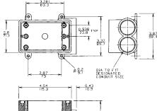
For multiple dead-end circuit terminations or where additional support is required in stub-up applications.
