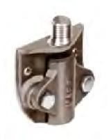
**NO. 690M**–A HEAVY DUTY VERTICAL POINT BASE FOR NO. 507 CABLE. THE TWO 1/4" CLEARANCE MOUNTING HOLES ELIMINATE THE NEED FOR ADDED POINT SUPPORT. THE 5/8" STUD ENGAGES ALL ADAPTER TYPE POINTS.
