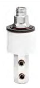
NO. 155AT—A THROUGH ROOF BASE WHICH ALLOWS FOR THE INSTALLATION OF A COMPLETE CONCEALED AIR TERMINAL BY ONE TECHNICIAN FROM ABOVE THE ROOF. THIS BASE REQUIRES AN ADEQUATELY SUPPORTED 1" PVC CONDUIT SLEEVE THROUGH THE ROOF. ROOF SEAL IS ACHIEVED VIA AN EPDM SEAL AND SOLVENT WELDED PVC PIPE CAP. IDEAL FOR USE WHERE AIR TERMINALS ARE CONNECTED DIRECTLY TO BUILDING STEEL. FOR CABLES THROUGH NO. 506.
