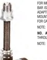
**NO. 709B**–A CONCEALED BASE AND RISER ASSEMBLY FOR METAL OR CONCRETE DECK CONSTRUCTION. RISER BAR IS  $\frac{1}{2}$ " DIAMETER BY 12". TOP ASSEMBLY FITS ALL ADAPTER TYPE AIR TERMINALS. THE PREMIUM DIE CAST MOUNTING BASE HAS A BOLT PRESSURE CABLE CLAMP FOR CABLES THROUGH NO. 506.
