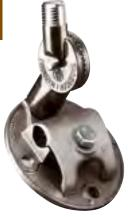
**NO. 30**-THIS PREMIUM DIE CAST BRONZE BASE INCLUDES A SWIVEL ADAPTER SO THAT POINTS MAY BE SET PERPENDICULAR ON A SLOPING ROOF. THE PREMIUM DIE CAST BOLT PRESSURE CONNECTION ACCEPTS CABLES THROUGH NO. 506. MOUNTING HOLES ARE ½" CLEARANCE. ORDER FASTENERS SEPARATELY.
