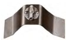
NO. 532—A HEAVY DUTY 31/4" WIDE, COPPER RAISED RIDGE SADDLE. BENDS TO FIT ANY ROOF SLOPE AND HOLDS POINT AND CABLE SLIGHTLY ABOVE THE CENTER OF THE RIDGE. PRESSURE TYPE CABLE CLAMP IS FOR CABLES THROUGH NO. 506. STUD ENGAGES ALL ADAPTER TYPE POINTS. (USE NO. 533 ATTACHMENT TO HOLD AND SUPPORT THE CABLE BETWEEN POINT LOCATIONS.)
