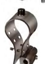
**NO. 240P-3**—A BIMETAL PLATED, CLAMP TYPE AIR TERMINAL BASE FOR MOUNTING ON PIPES, ROUND HANDRAILS, ETC. UP TO 11/4" O.D. HAS INTERNAL THREAD FOR 3/8" LESS ADAPTER TYPE POINTS. (CLASS I ONLY.)
