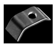
NO. 168-A 5/8" WIDE HEAVY DUTY SOLID COPPER CLIP WITH SLOTTED MOUNTING HOLE FOR 1/4" MAXIMUM FASTENERS. CLIP ACCEPTS A WIDE RANGE OF CONDUCTORS FROM NO. 14 THROUGH NO. 507.
