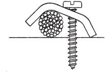
**NO. 167**–A  $\frac{1}{2}$ " WIDE COPPER CLIP SIMILAR TO NO. 168 FOR MOUNTING WITH NAILS OR OTHER FASTENERS NOT OVER  $\frac{3}{6}$ " DIAMETER.
